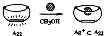
Scheme 3 Fluorescence quenching by complexation in craterophane A22
